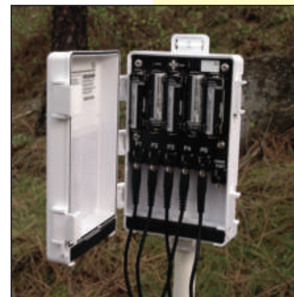
▲ Em50 loggers provide a turn-key solution for the ECH 2 O probes.
