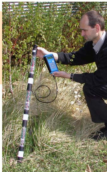
Multilevel Tensiometer with three modules: soil water tension is measured in depths of 90 cm, 60 cm and 30 cm.
